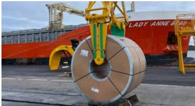
Spreader for steel coils
