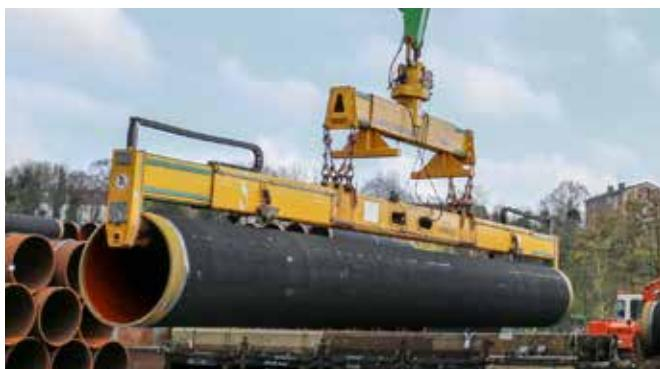
Quick change system with lifting beam
