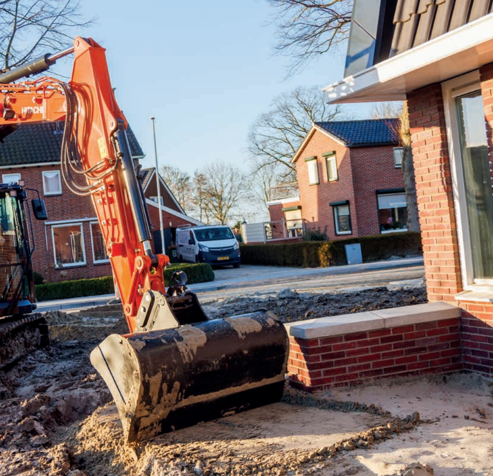
Short distance between the bucket and blade enhances efficiency and safety.
