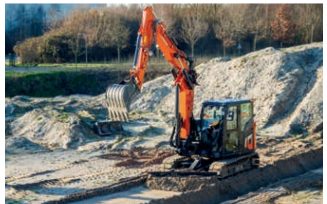
The optional floating angle blade is ideal for grading and levelling.
