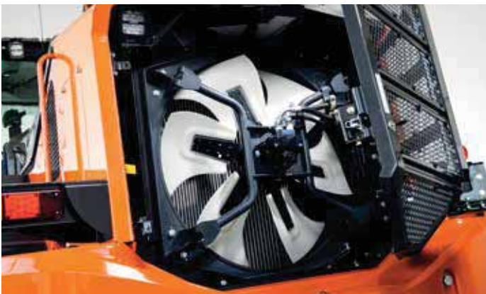
Intelligent fan operation system prevents radiators clogging.
