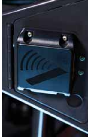
Rear obstacle detection system enhances safety on the job site.
