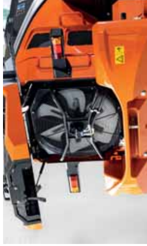
Intelligent fan operation system prevents radiators clogging.
