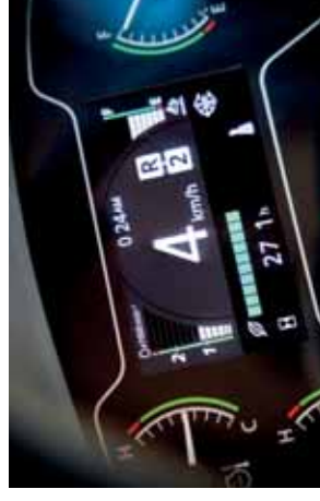
The ECO gauge helps to deliver better fuel consumption.
