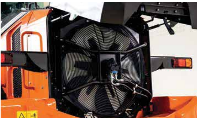
Intelligent fan operation system prevents radiators clogging.
