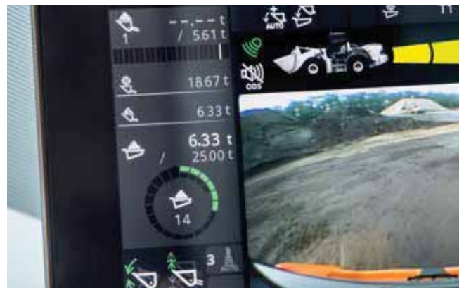
Work more productively and accurately using the payload checker.
