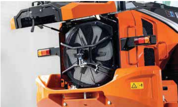
Intelligent fan operation system prevents radiators clogging.
