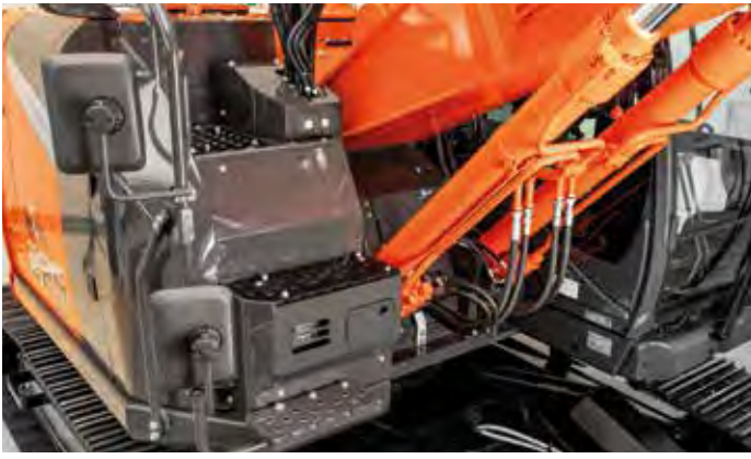
Wide steps on the ZX225US/USR-7 allow for easier maintenance.
