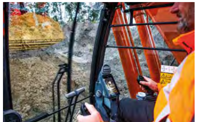
Wider wiper design provides greater visibility.
