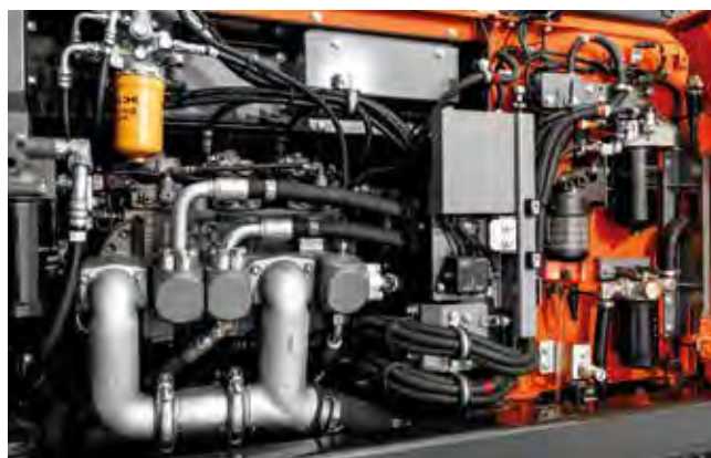
A fuel saving of up to 11% is achieved with the TRIAS III hydraulic system.
