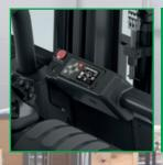
Onboard preoperation checklist and overload alarm. An interactive truck with a safe operation indicator. Fully automatic parking brake with anti-rollback function.
