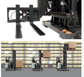
**Simultaneous access to both sides of the aisle** With the 180° Swivel Reach fork unit, the operator conveniently rotates the forks to allow placement of goods into the racking on either side of the aisles – instead of turning the truck, the operator turns the forks.
