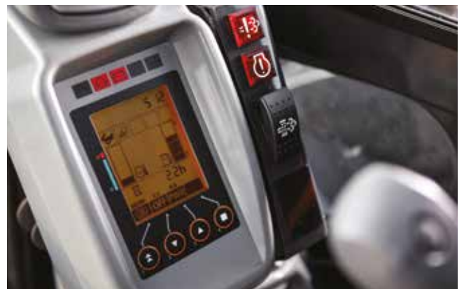
Multifunctional LCD monitor shows data at a glance.
