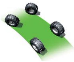
FRONT WHEEL STEERING MODE
