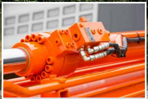
Hose rupture valves for arm and boom guarantee a safe lifting operation.
