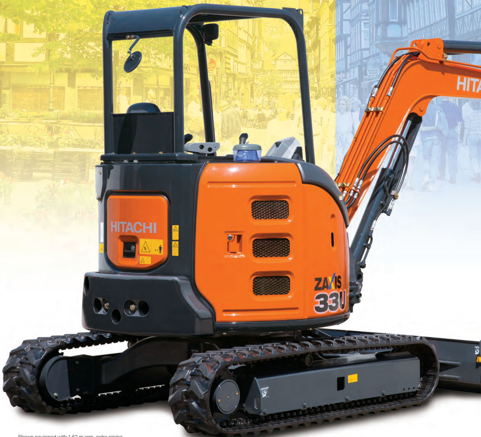
Shown equipped with 1.52 m arm, extra piping, additional counterweight, rear view mirror, armrests, and pre-cleaner.
