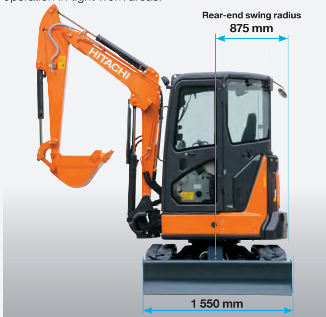
Shown equipped with 1.52 m arm, extra piping and additional counterweight.
