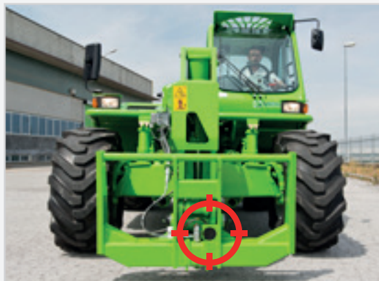
Sensor on the carriage
