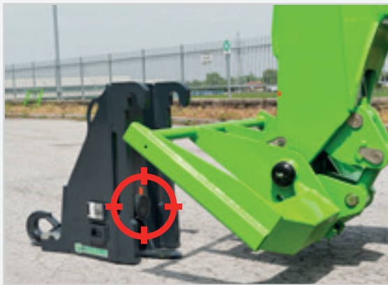
Sensor on the attachment
