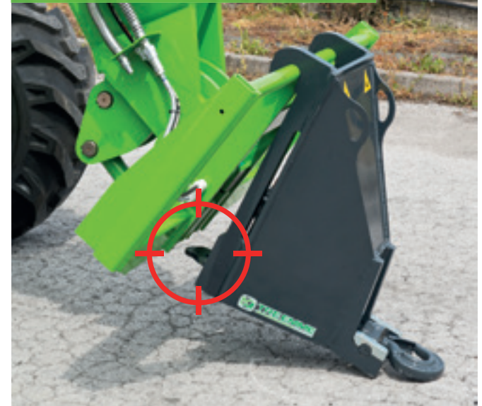
Tac-Lock: hydraulic attachment clamping system from the cab
